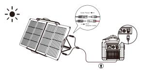
This cable can only be used for connection between solar panels and energy storage. It is prohibited to be used for interconnection between solar panels or other connection purposes.
