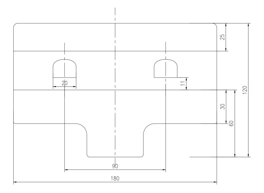
Measure Unit: mm Material: Anti UV ABS Color: Black/White Overall Length: 180mm
